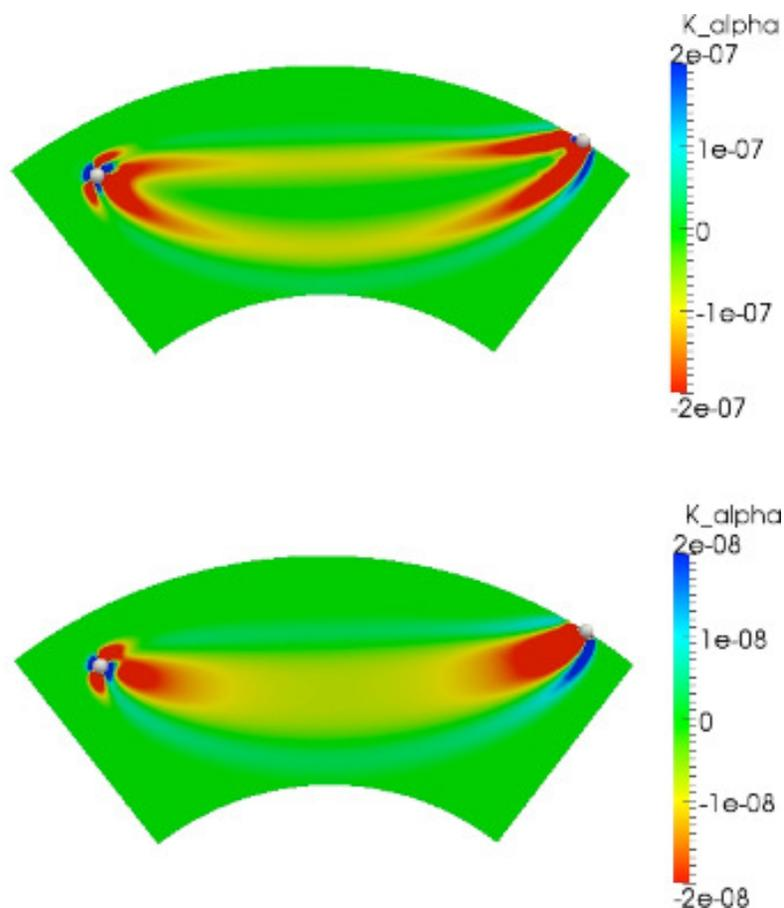
Figure 10.2: P-wave speed finite-frequency kernels from cross-correlation travelttime (top) and amplitude (bottom) measurements for a P arrival recorded at an epicentral distance of  $60^\circ$ . The kernels together with the associated files and routines to reproduce them may be found in `EXAMPLES/global_PREM_kernels/`.
