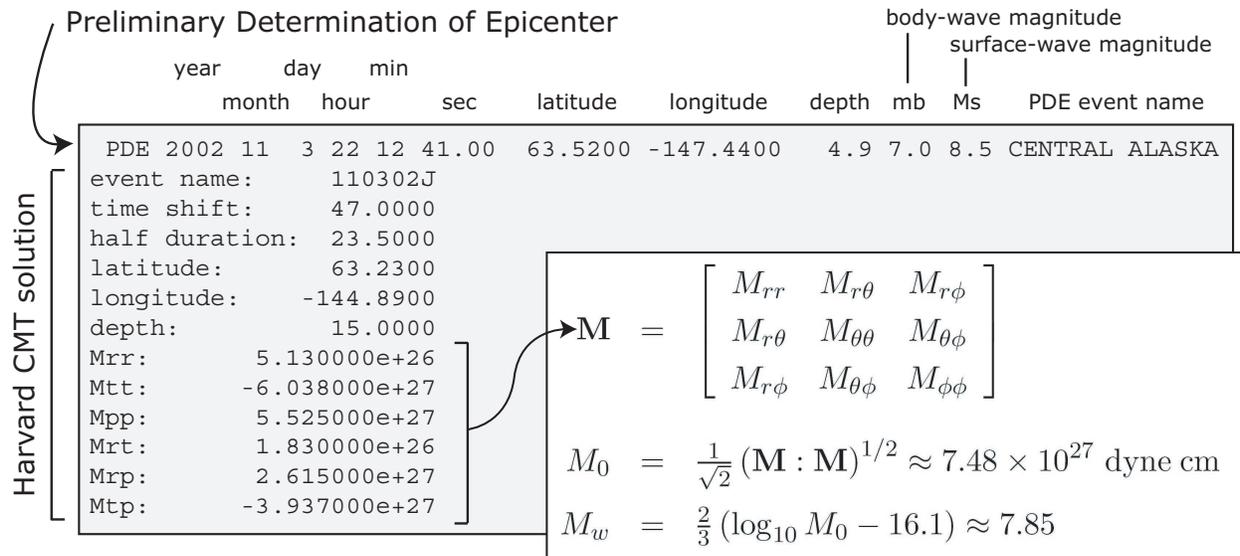
Figure 4.1: CMTSOLUTION file obtained from the Harvard CMT catalog. The top line is the initial estimate of the source, which is used as a starting point for the CMT solution.  $\mathbf{M}$  is the moment tensor,  $M_0$  is the seismic moment, and  $M_w$  is the moment magnitude.
