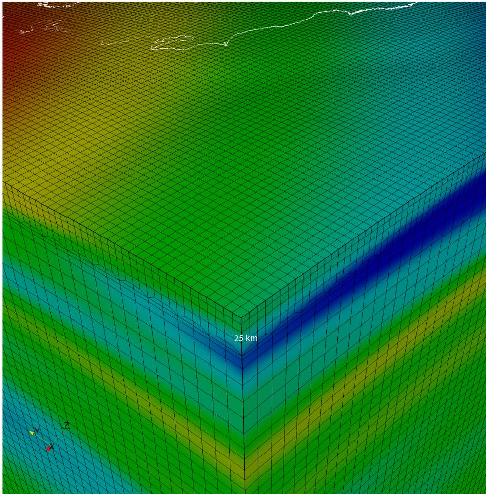
Figure 5.2: Close-up view of the upper mantle mesh shown in Figure 5.1. Note that the element size in the crust (top layer) is  $13 \text{ km} \times 13 \text{ km}$ , and that the size of the spectral elements is doubled in the upper mantle. The velocity variation is captured by  $\text{NGLL} = 5$  grid points in each direction of the elements [Komatitsch and Tromp, 2002a,b].
